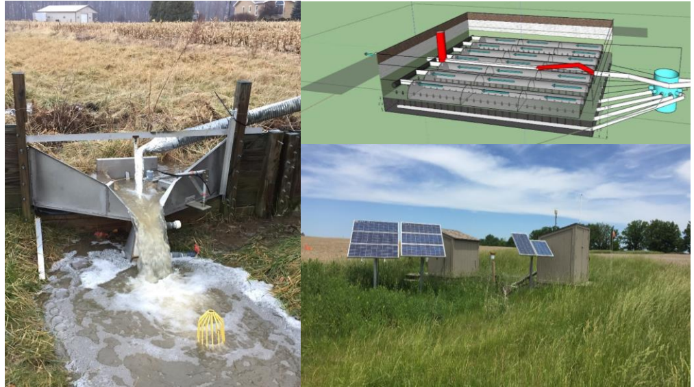
Clockwise from left: Measuring surface runoff from an edge-of-field plot; In-field phosphorous removal structure designed to treat surface and subsurface flows; Water quality monitoring site infrastructure.
